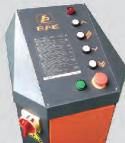
24v Safe Control System
