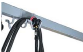
Hanging rack with tools,grinding tools can hang buy to temporarily not work, clean and orderly
