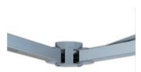
2.5m+2.5m working arm cover two station, two people can be grinding at the same time
